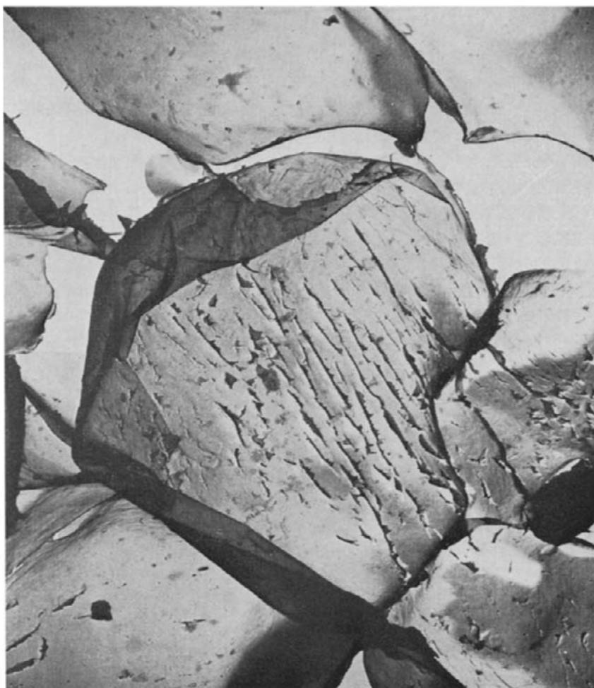
Fig. 8. Surface replica of partially decomposed cobalt malonate (salt B, \alpha = 0.30 ). ( \times 7,000 .)
